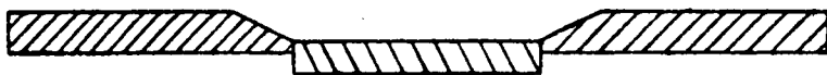
FIG. 1. Section of early type of roller table with concave door and no batters.
