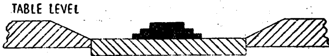
FIG. 13. The same octagonal arrangement as shown in Fig 12, but fitted below table level
