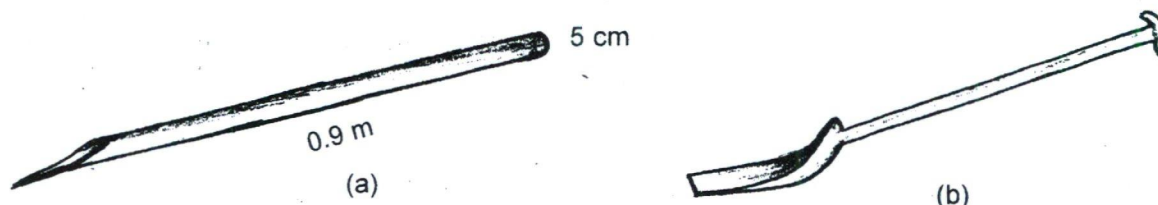
Figure 1. A diagrammatic sketch of a sampling probe (a) and a shovel (b)
