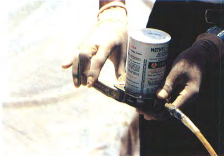
Plate 0 2- MeBr can is fitted into the groove in the Jiffy Applicator When the lever held by the right hand is turned inwards it pierces the can releasing the liquefied gas which flows out through the tube
