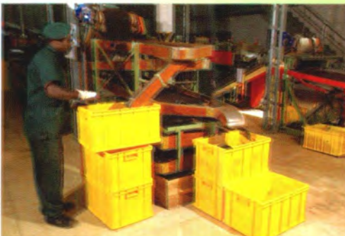
Chota-Rotary sifter(grading of tea)
