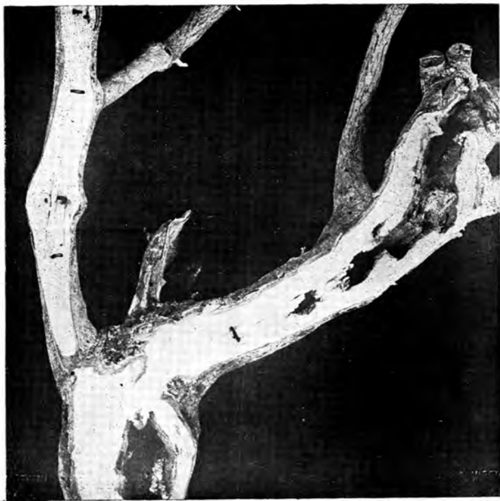
FIGURE 7.—An example of advanced internal wood rot, showing cavities cleared out and gradually enlarged by scavenging termites. ( see also figure 35)
